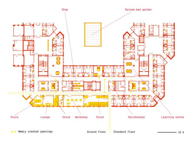
Partial plan of Haus Erdberg, Standard floor with shops in the central areas. The ground-floor workshop is shown in the detailed excerpt.
